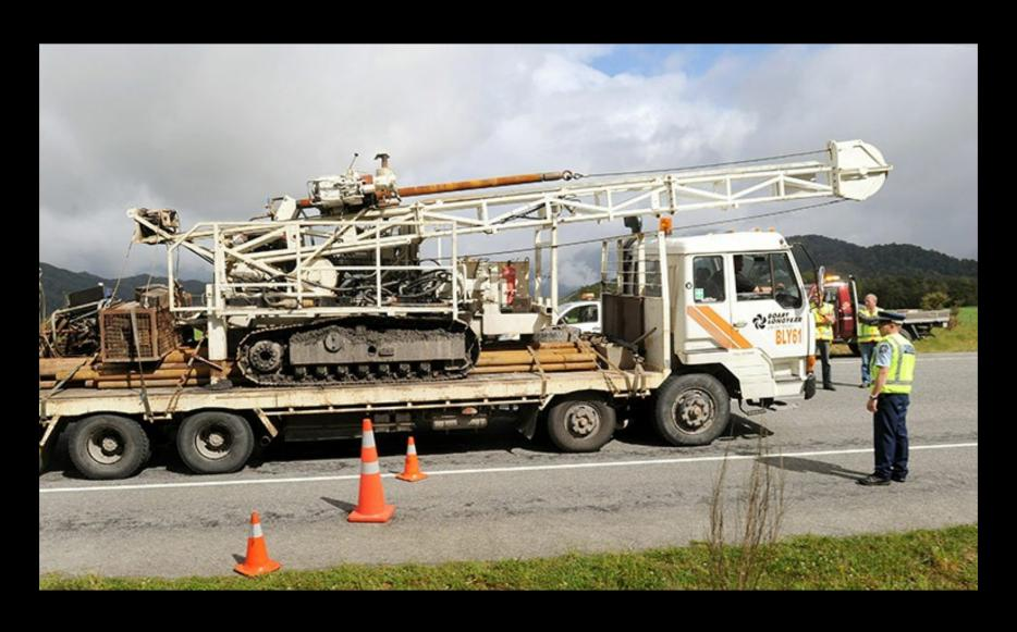
Sampling borehole drill rig
