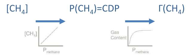
An adsorption isotherm is needed to calculate gas content from CDP
