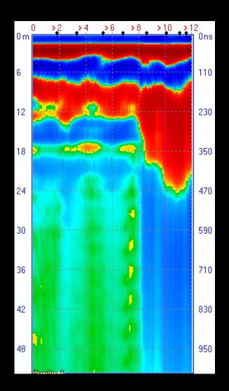
Paleo channel (red) to 26m depth cutting and destroying the coal resource - 6m thick coal seam from 12m and 18m depth.
