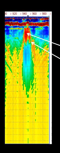
Vertical Dyke (~2m thick) known from ground magnetic survey.
