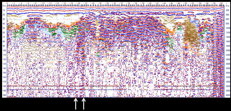
Voids from 2 sub vertical, open drill holes. No steel casing. Left hole depth = 140m. Right hole depth >200m. Left dip on Left hole is real. Filter was optimised for target strata not drill holes!
